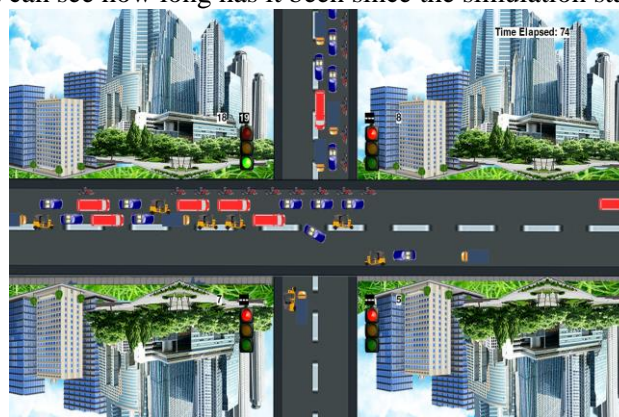
Figure 4: The simulation begins with red and green lights, with the green signal timer having By default, the red signal timer is blank and the countdown starts at 20. We display an empty value for 10 seconds when the signal is red. The count of vehicles that have passed through the signal can be seen next to it, which is initially all zero. On the top right, you can see how long has it been since the simulation started?
